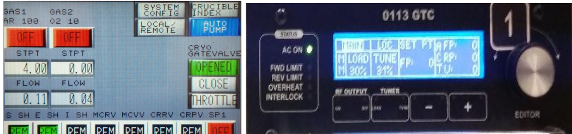
Main Menu, ProFace, L, showing gas, and RF Generator, R, for Back sputtering
