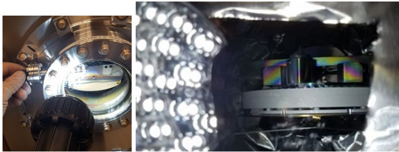
Above: shadow fixture, marking screw, 3 different pieces, sample holder placed when fixture is loose, to allow loading room, then tightened last.
