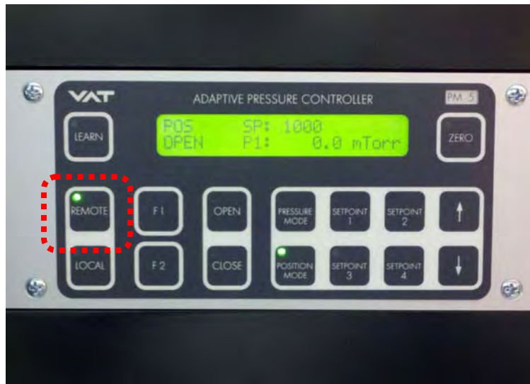
Figure 12 Chamber pressure controller
