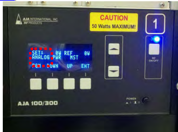
Figure 16 Sample bias RF generator
