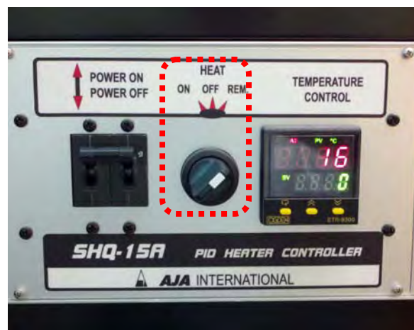
Figure 13 Substrate heater controller
