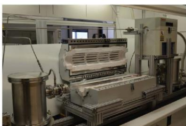
Figure 1: Split zone CVD reactor for roll to roll production of 2D materials.
