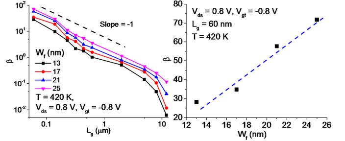
Fig. 9. Left:  $\beta$  (log-log scale) versus  $L_g$  for devices with different  $W_f$ . Right: Current gain as a function of  $W_f$  for  $L_g = 60 \text{ nm}$ .
