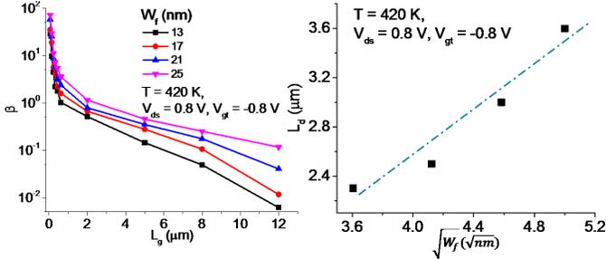
Fig. 8. Left:  $\beta$  as a function of  $L_g$  for different  $W_f$ . Right: extracted  $L_d$  versus  $\sqrt{W_f}$  revealing a linear dependence.
