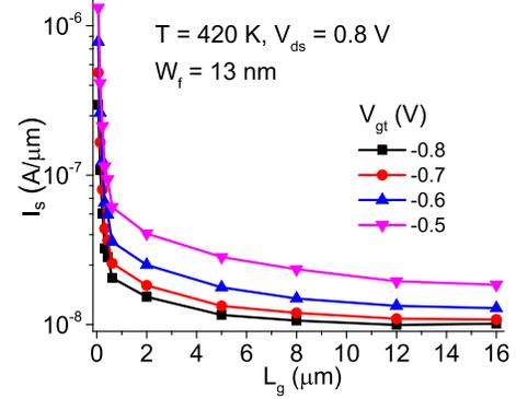
Fig. 6. Source current of  $W_f = 13$  nm,  $N_f = 34$  FinFETs with various  $L_g$ , showing saturating OFF-state current for  $L_g > 8 \mu\text{m}$ . This is the pure BTBT current.
