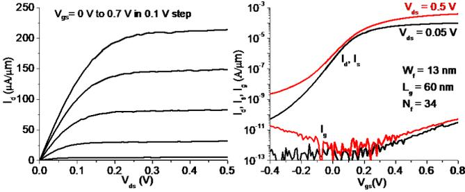
Fig. 2. Output and subthreshold characteristics of an InGaAs FinFET with  $W_f = 13$  nm,  $L_g = 60$  nm, and  $N_f = 34$ .
