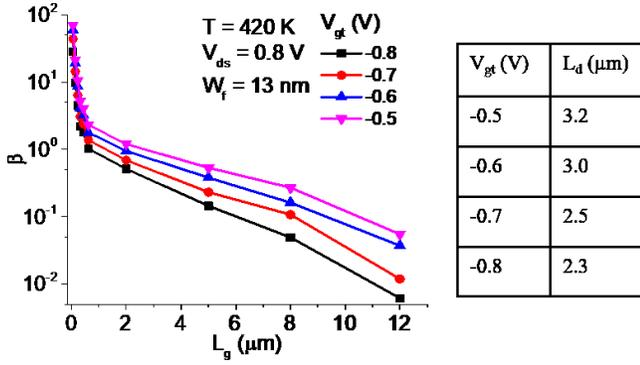
Fig. 7. Bipolar gain as a function of  $L_g$  for the device in Fig. 6 in the semilog scale (left). Extracted electron diffusion length ( $L_d$ ) in the channel (right table).
