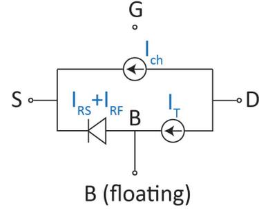
Fig. 3. Equivalent circuit diagram for off-state current.
