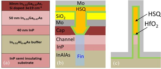
Fig. 1. (a) Starting heterostructure, (b) cross-sectional schematic along with the fin length, and (c) across the fin width in a finished device. In (b), the blue region indicates the location of the fin.
