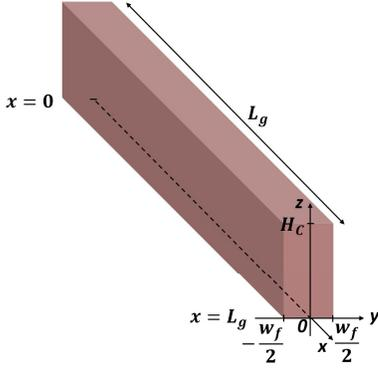
Fig. 4. Schematic showing the fin geometry.
